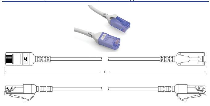
Stranded bare copper conductors insulated with thermoplastics polyolefin. Two insulated conductors twisted together to form a pair and four such pairs cabled to form the basic unit. Overall jacket with LSZH. Unique tight extrusion for up to 30% reduction in diameter.
