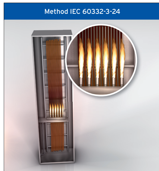
A cable bundle is exposed to a line of flames for 20 minutes in a 4 meter high cabinet. Approximately one meter above the flames the cable bundle must extinguish itself with only a minimal production of smoke.
